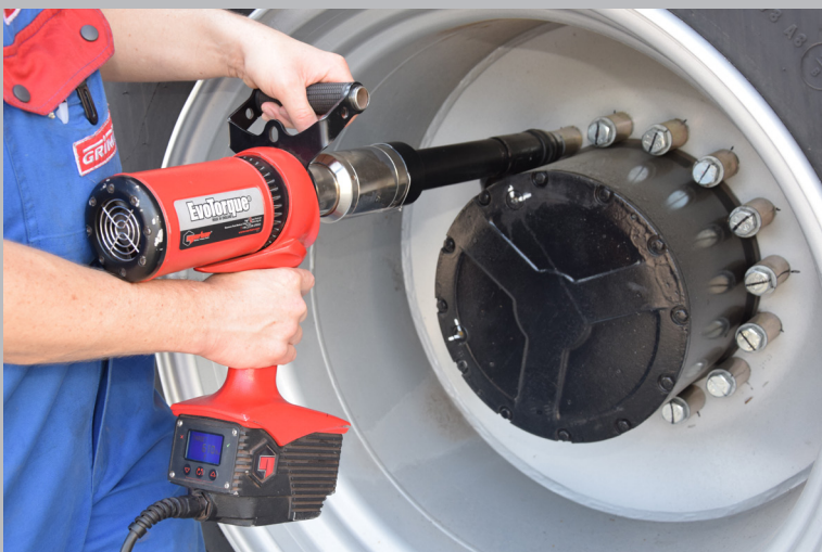
EvoTorque fitted with 12" nose extension performing its bolting operation
